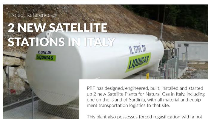
water exchanger and a cryogenic pump-equipped LNG transfer skid, so that the LNG can be discharged, and then transported in ISO containers by land or sea.
